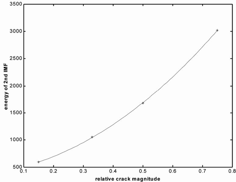
Figure 4: Energy of 2<sup>nd</sup> IMF as a function of relative crack magnitude.
