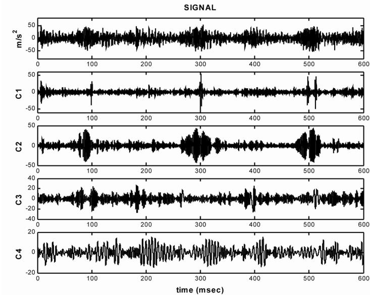
Figure 2: Decomposition of the vibration signal into intrinsic mode functions.
