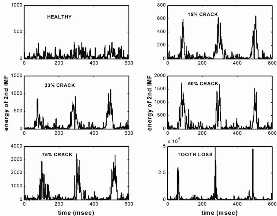
Figure 3: From top to bottom, energy of 2<sup>nd</sup> IMF for a healthy gear pair, a pair with 15%, 33%, 50%, 75% crack and tooth loss.
