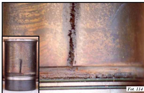
Figure 4: Cavitation erosion with removal of further material layers in wet-sleeve liners was observed after 1500 working hours. It is about a turbocharged engine with 6 cylinders of bore x stroke = 105 x 115,5 mm, in the cooling system of which anticorrosion and anticavitation inhibitors had been used.
