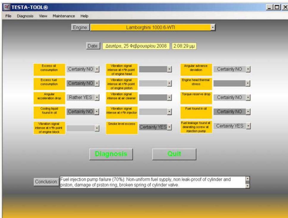
Figure 8: Demonstration of TESTA\_TOOL diagnostic capabilities
