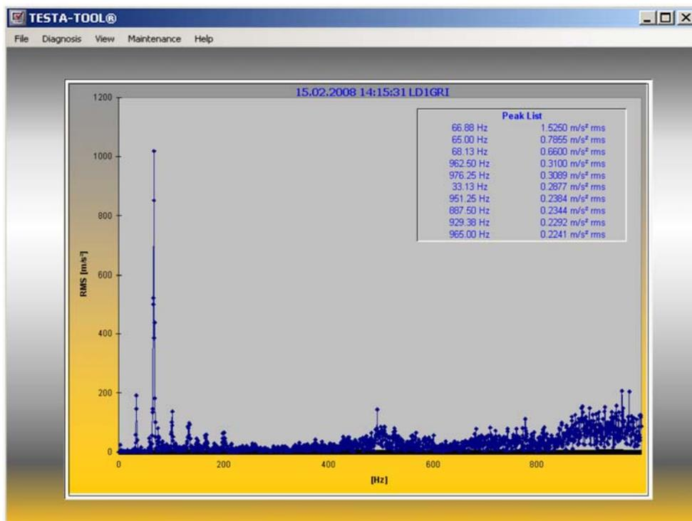
Figure 6: Example screen with recorded graph of the vibration FFT spectrum at n<sup>th</sup> point of the engine block (Lamborghini 1000.6-WTI)
